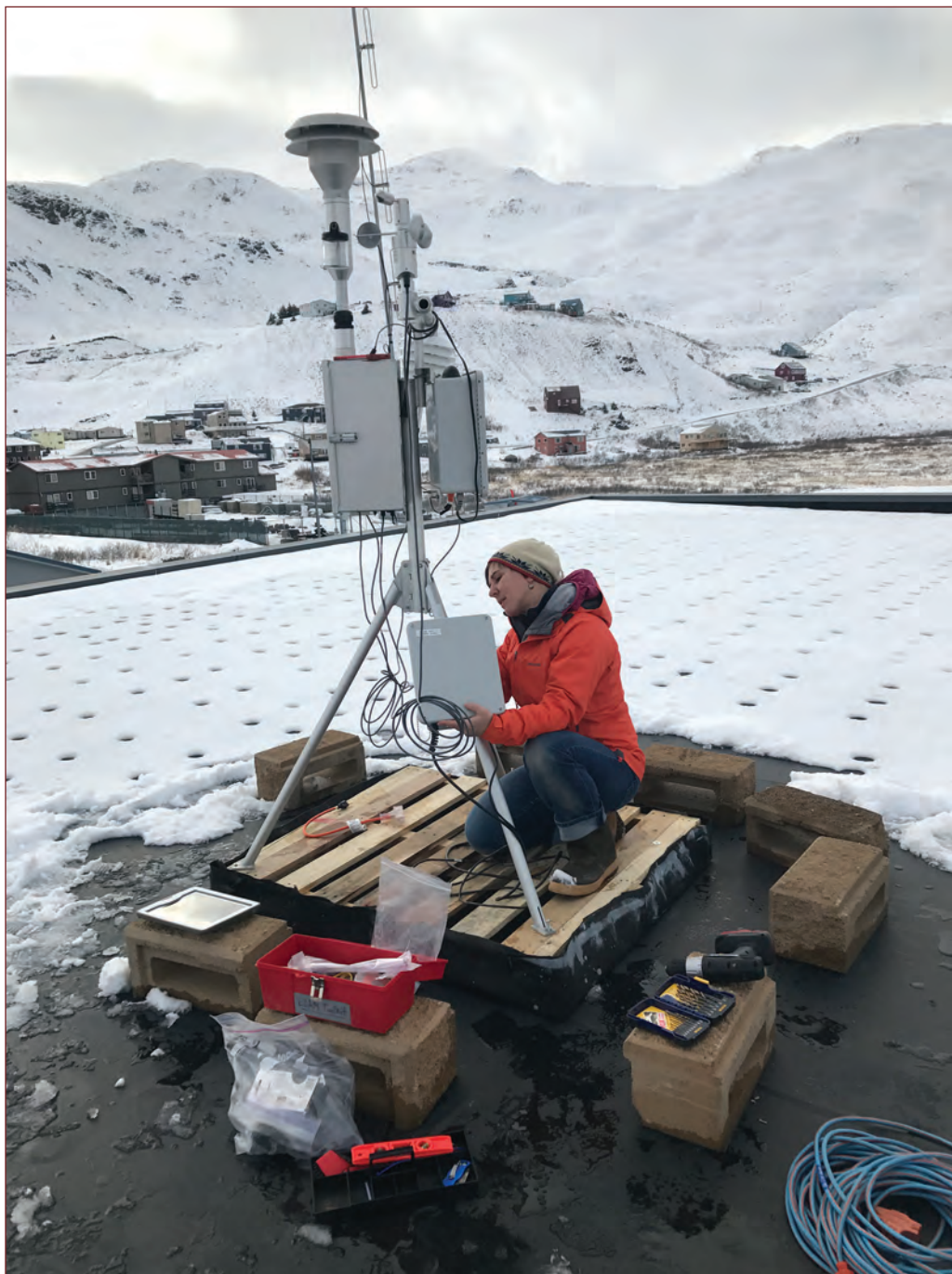
A U.S. Geological Survey scientist installs an air-quality monitor in Unalaska, Alaska, during the eruption of Bogoslof Volcano in February 2017. Alaska Volcano Observatory/U.S. Geological Survey photograph by Janet Schaefer.
