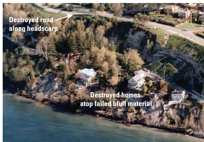
Figure 5. Landslides in Seattle, Washington. These photos of typical landslides along Seattle's coastal bluffs illustrate that subduction zone hazards don't only manifest as infrequent, major catastrophes to entire communities; they also impact lives, property, and infrastructure regularly in smaller, but still locally significant, events. Deep-seated slides, like the one shown in the left photograph, involve movement of large masses originally rooted in bedrock or relatively old sediments (photograph by L. Palmer, Federal Emergency Management Agency). In shallow slides, like the one shown in the right photograph, soils and younger sediments often rapidly flow downhill (photograph copyright 1997, T. Tamura, Seattle Times).
