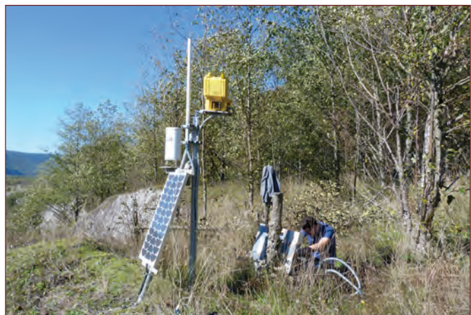
A technician installs lahar monitoring equipment in Washington State. U.S. Geological Survey photograph by Elizabeth Faust.
