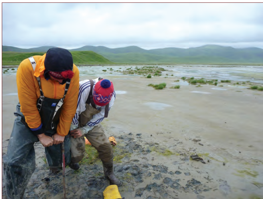
Geologists drive a core into marsh sediment to document interbedded peat and silt that records sudden vertical land movements associated with fault slip during large subduction-zone earthquakes. U.S. Geological Survey photograph by Rich Briggs.
