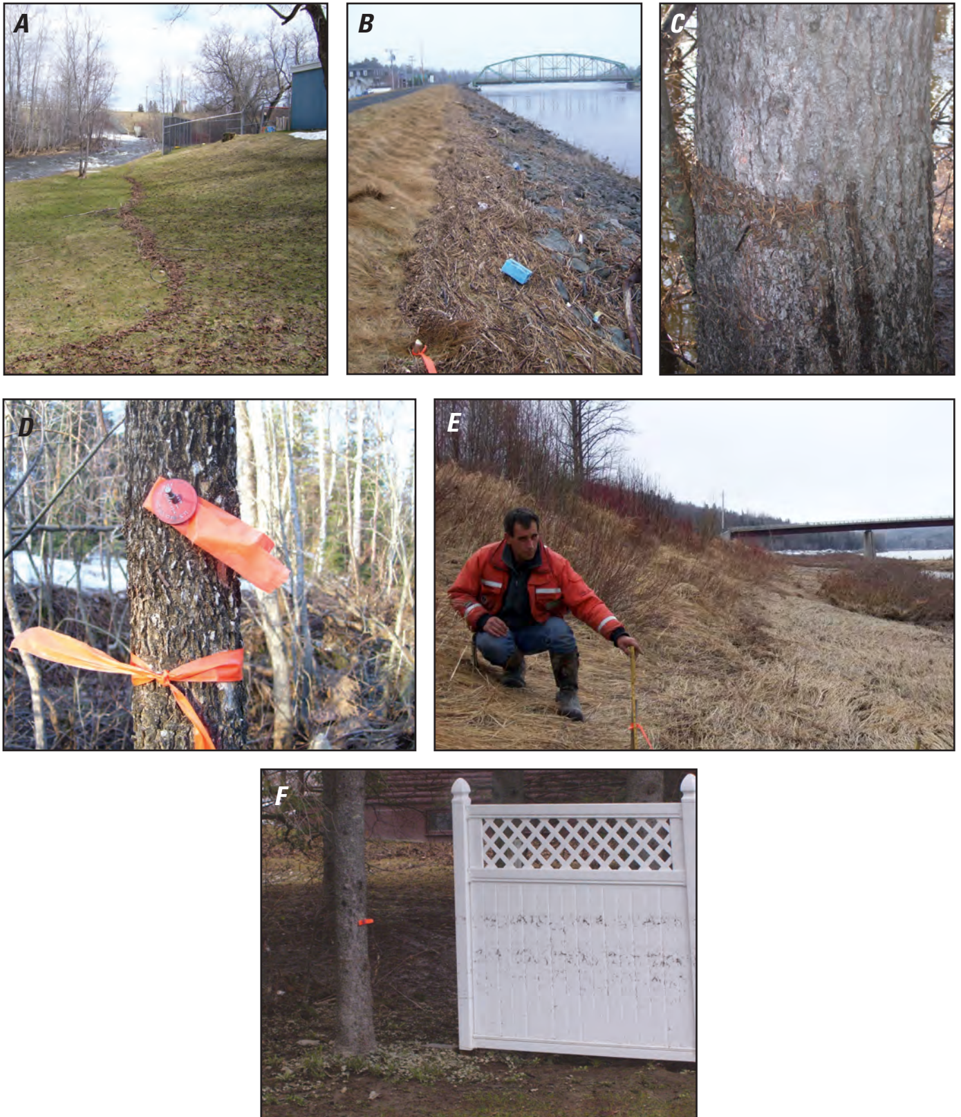
Figure 8. High-water mark identification and marking after the April/May 2008 flood in northern Maine: (A) debris line, (B) debris line along St. John River dike in Fort Kent looking downstream at International Bridge, (C) debris line on tree, (D) U.S. Geological Survey high-water marker, (E) setting high-water mark along St. John River in Allagash, and (F) debris line on fence in Fort Kent. (Photographs by Laura Flight and Andrew Cloutier, U.S. Geological Survey)
